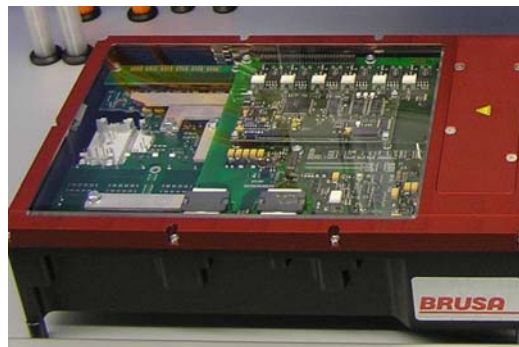
40kW SoftSwing® inverter with softPHASE modules from Tyco Electronics
