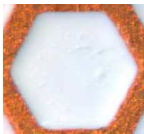
Fig.2.17: Skin effect on thermal paste
