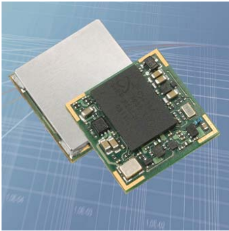
The A1084 modules of SiRFstarIII-based GPS receivers which supports both passive and active antennas.
